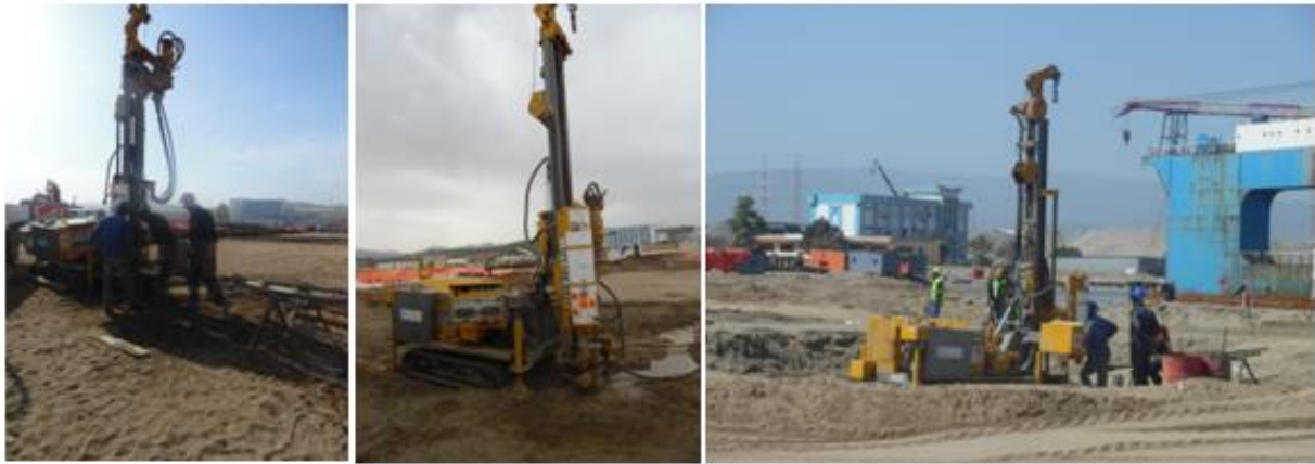
Figure IV. 8: (a) Photographs of the SPT test [57].
