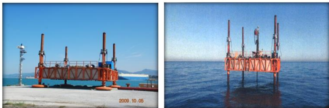
Figure II. 3: SPT testing equipment loaded onto a offshore floating barge [51, 52, 54].
