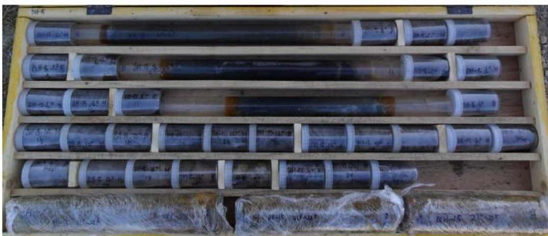
Figure II. 5: (b) Undisturbed samples collected during standard penetration for soil classification and physical characteristics tests [55].
