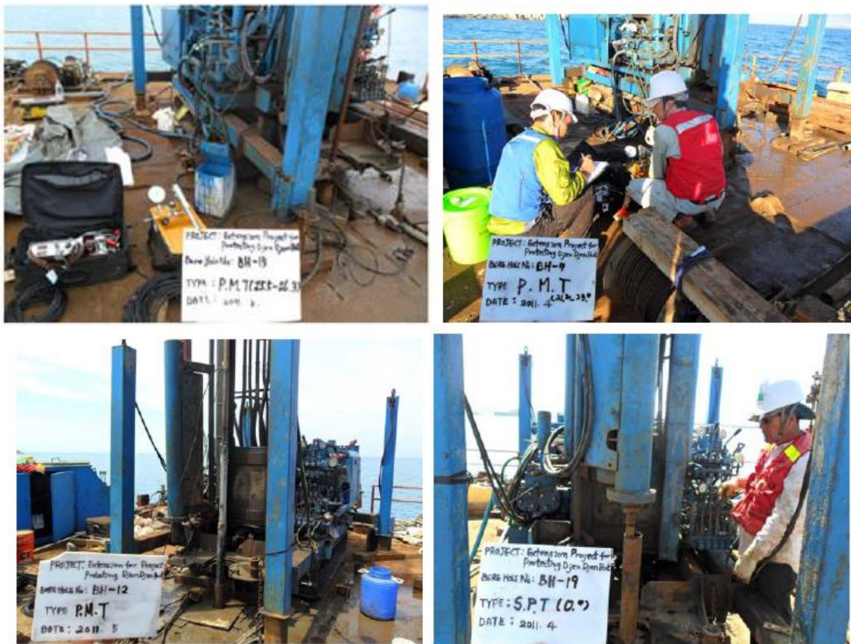
Figure II. 4: Photography of SPT testing equipment loaded onto a offshore floating barge [54].
