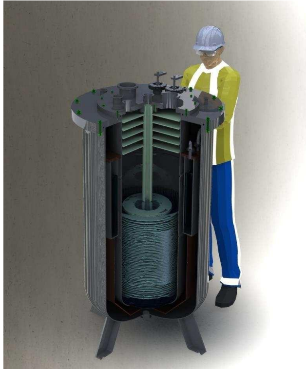
Figure 92: Representation of the SMES in its cryostat [Courtesy SigmaPhi®].
