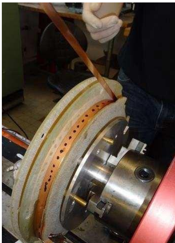
Figure 98: Gluing of the last turns of the pancake with Stycast®.
