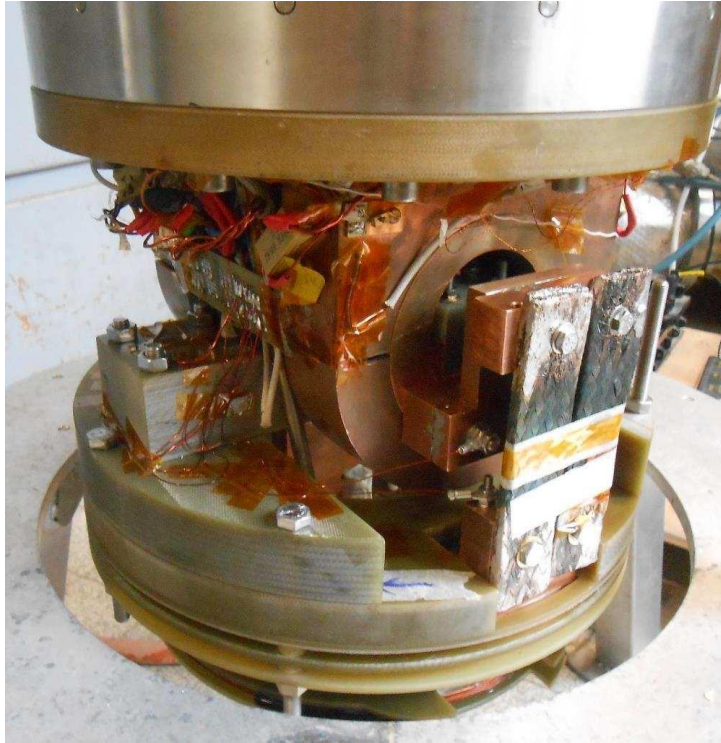
Figure 123: The pancake and its compensation coils mounted on the 3 kA EuCARD probe (see part III-1.1). The extensions of the contacts are connected to the current leads of the probe by copper braids, which enables the connection to be partially flexible. This mounting is also visible in Fig. 104.b.
