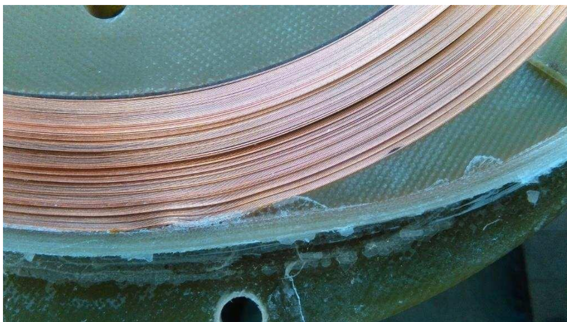
Figure 117: View of the first pancake after dismounting of the external flange. The deformation of the pancake due to the centripetal pressure of the bracing is clearly visible.
