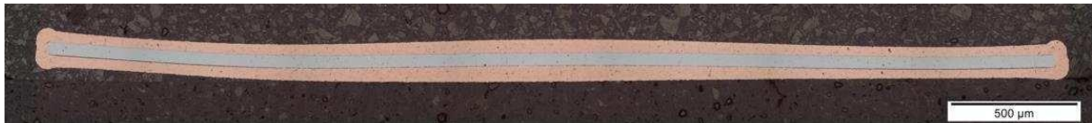
Figure 85: Cross section of a REBCO tape with irregular copper deposition.
