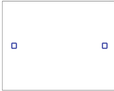
Figure 72: Aspect ratio of a solenoid with a=0.06 and \$=0.106 . This topology maximizes the specific energy of a solenoid with J = 500 \text{ A/mm}^2 , E = 20 \text{ MJ} and having a hoop stress (calculated by the Wilson formula) lower than 800 \text{ MPa} .
