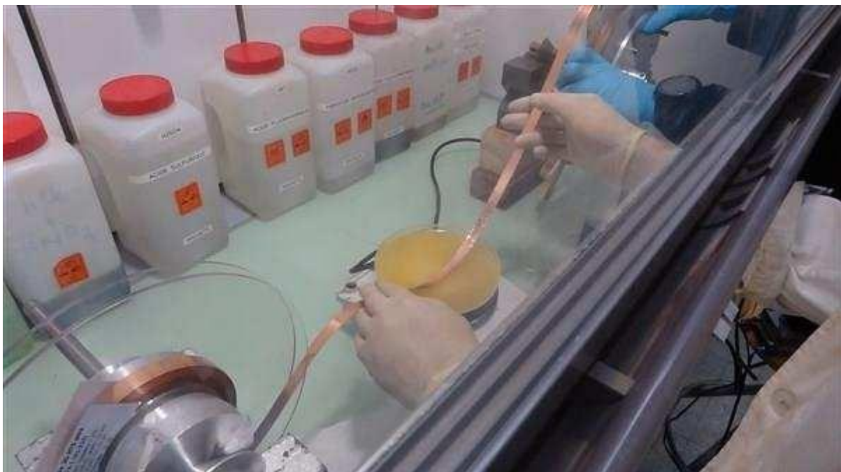
Figure 97: Operation to remove the insulation from the tape, in order to solder the tape to the external contact.
