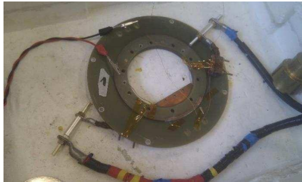
Figure 112: Measure of resistivity of an inner contact, immersed in liquid Nitrogen.
