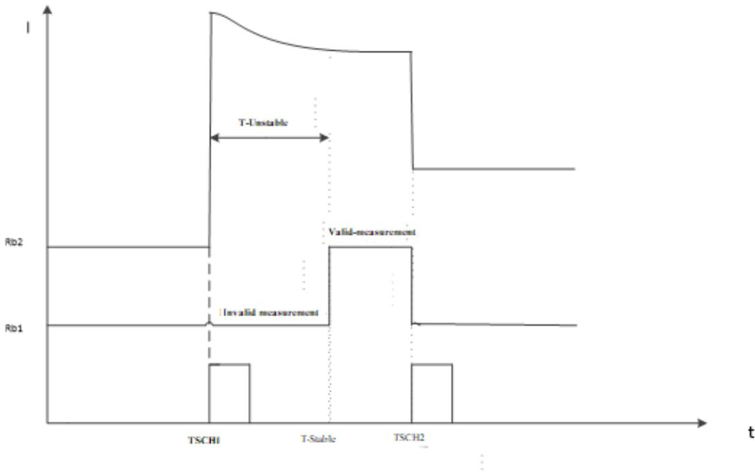
Fig. 5.1: The variable load measurement
