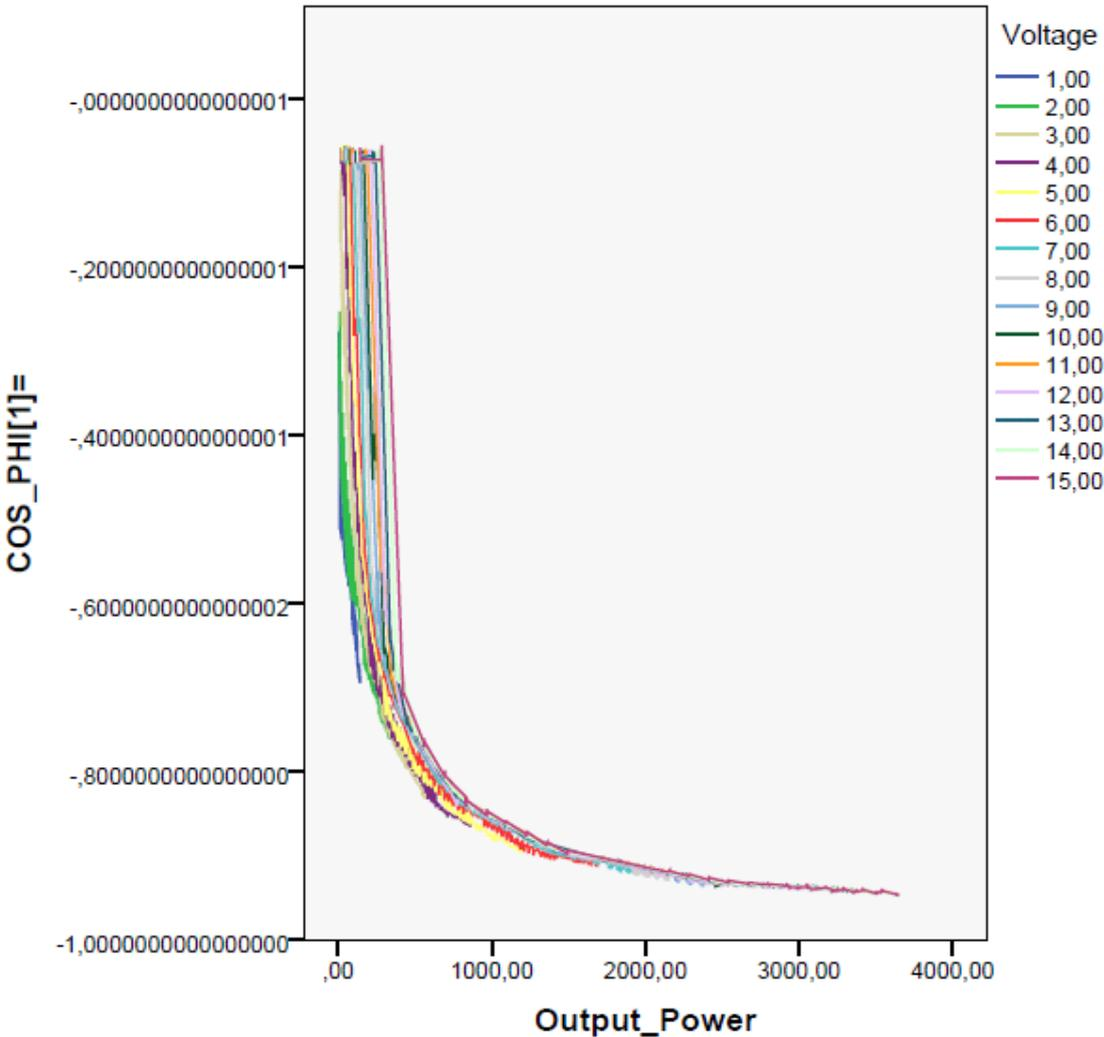
Fig. I.3: The output power(W) vs Cos phi
