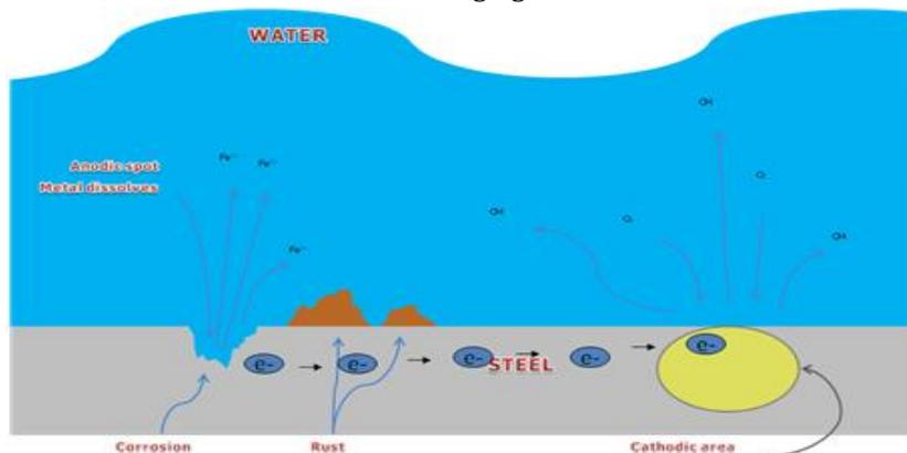
Fig. 1.3: Metal without ICCP protection
