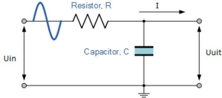
Fig. 6.4: Low pass filter circuit
