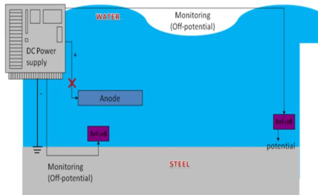
Fig. 1.5: Cathodic protection by impressed current
