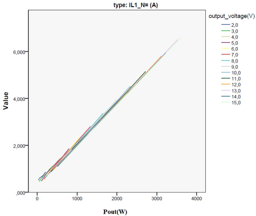
Fig. G.8: I fase vs Puit for phase 1
