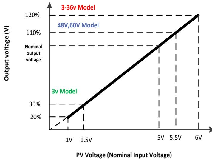
Fig. 3.5: Linear output against the PV voltage
