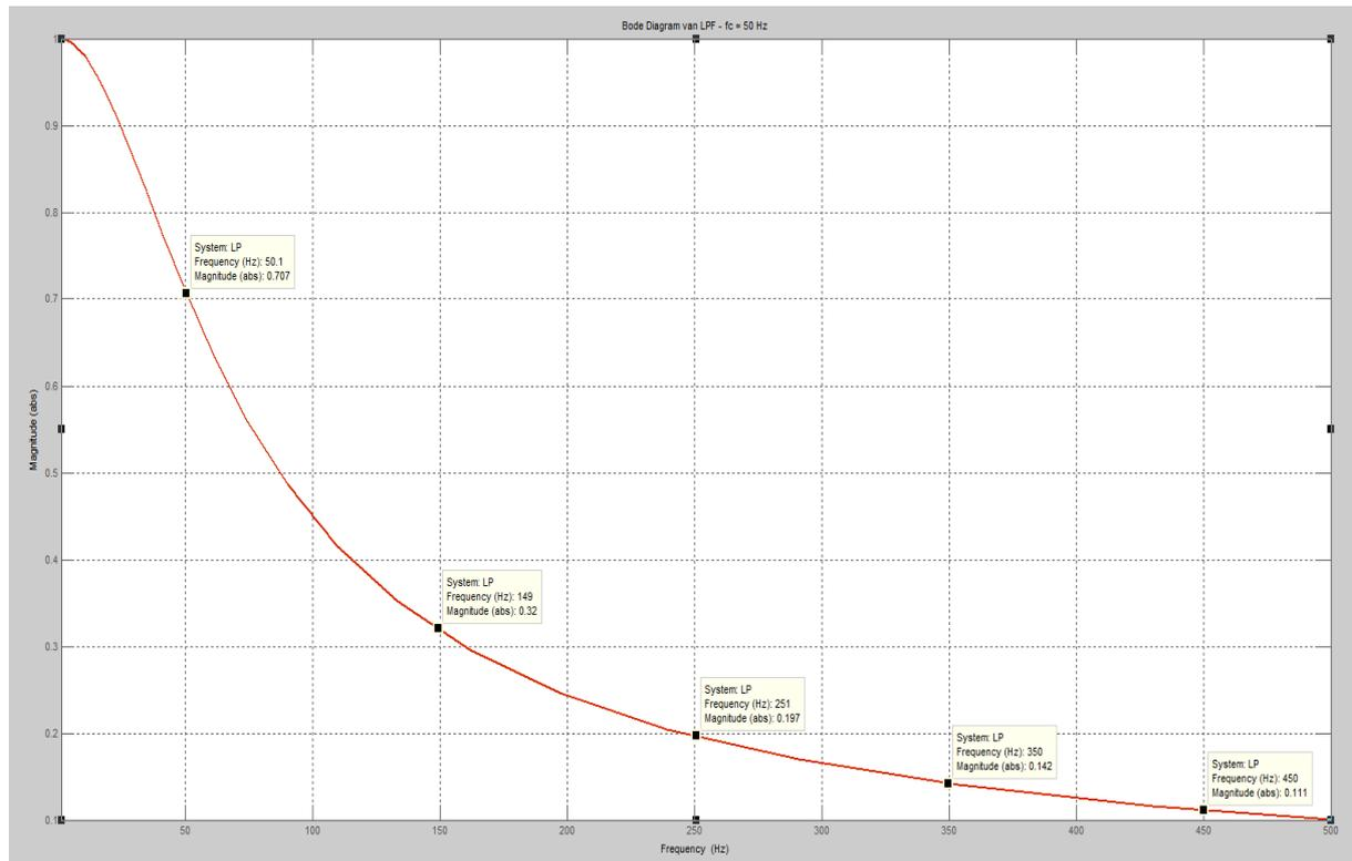
Fig. 6.8: Bode diagram of LPF - fc=50 Hz
