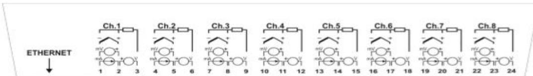
Fig. 4.4: The bottom connections of the FieldLogger
