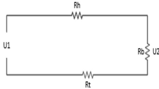
Fig. 4.36: The voltage divider of R cable and R load
