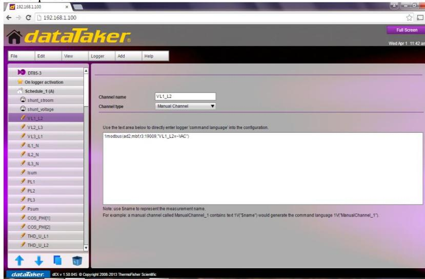
Fig. 4.17: Modbus address of phase voltage
