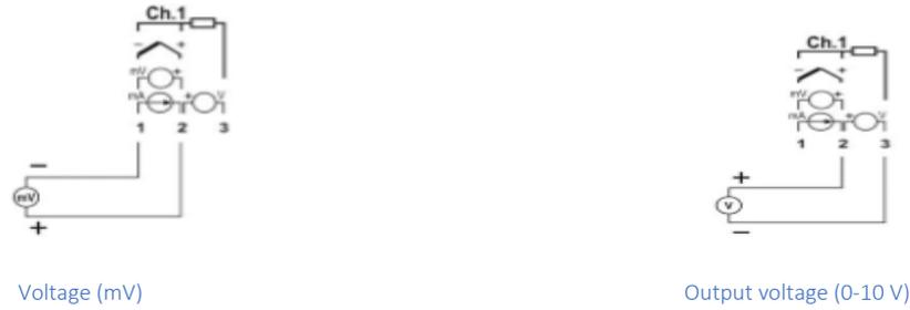
Fig. 4.6: Analog Inputs - Connection
