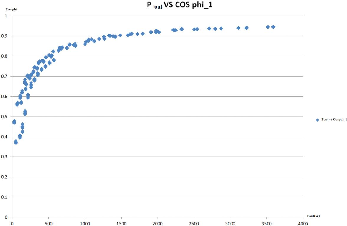
Fig. G.3: The power output VS Cos phi
