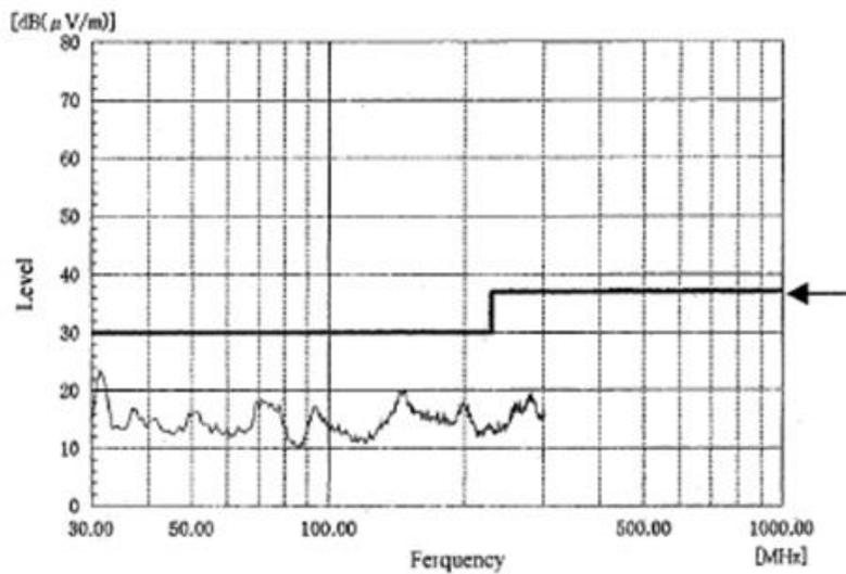
Fig. C.2: Electric magnetic interference properties for HWS 1000-15
