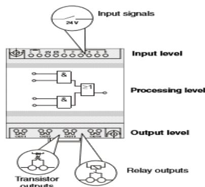
Fig. 4.22: The principle of information processing
