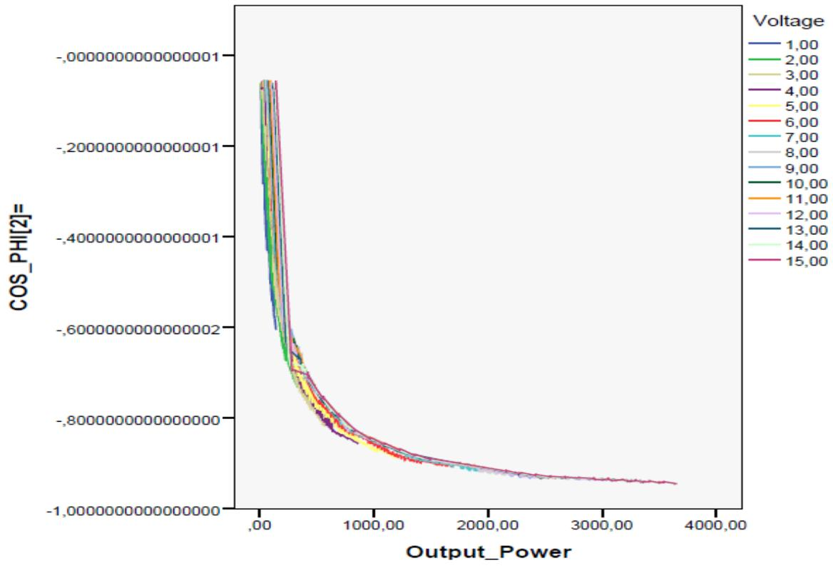
Fig. I.9: Output power vs cos phi of phase 2
