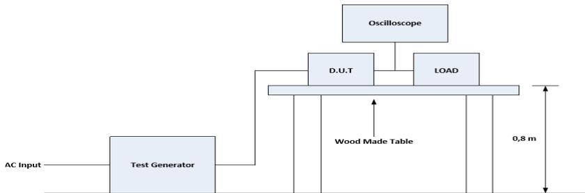
Fig. B.2: Voltage dips, short interruption, immunity test
