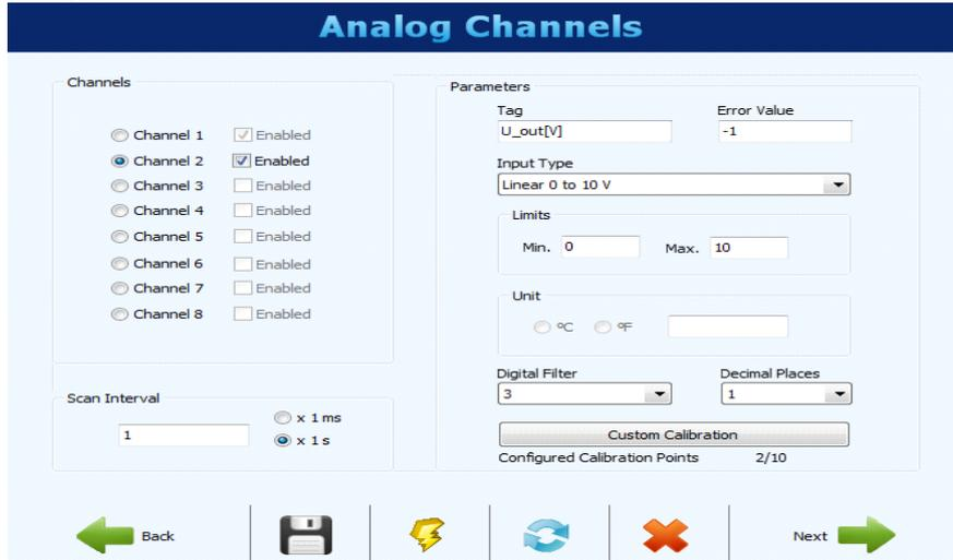
Fig. 4.9: Analog Channels Configuration- Output Voltage
