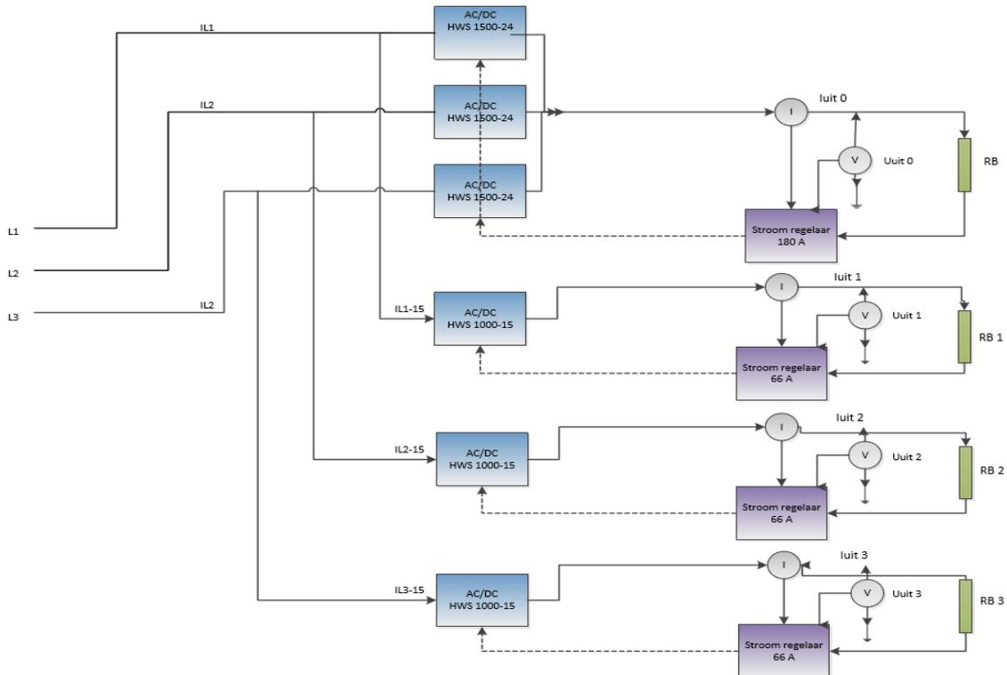
Fig. 5.5: ICCP controller block diagram
