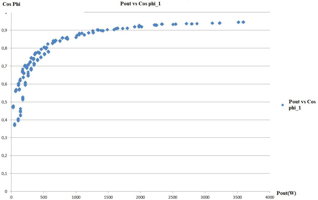
Fig. H.2: Pout vs Cos phi for Phase 1
