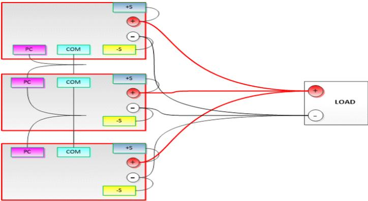
Fig. 3.3: Connected parallel AC / DC converters
