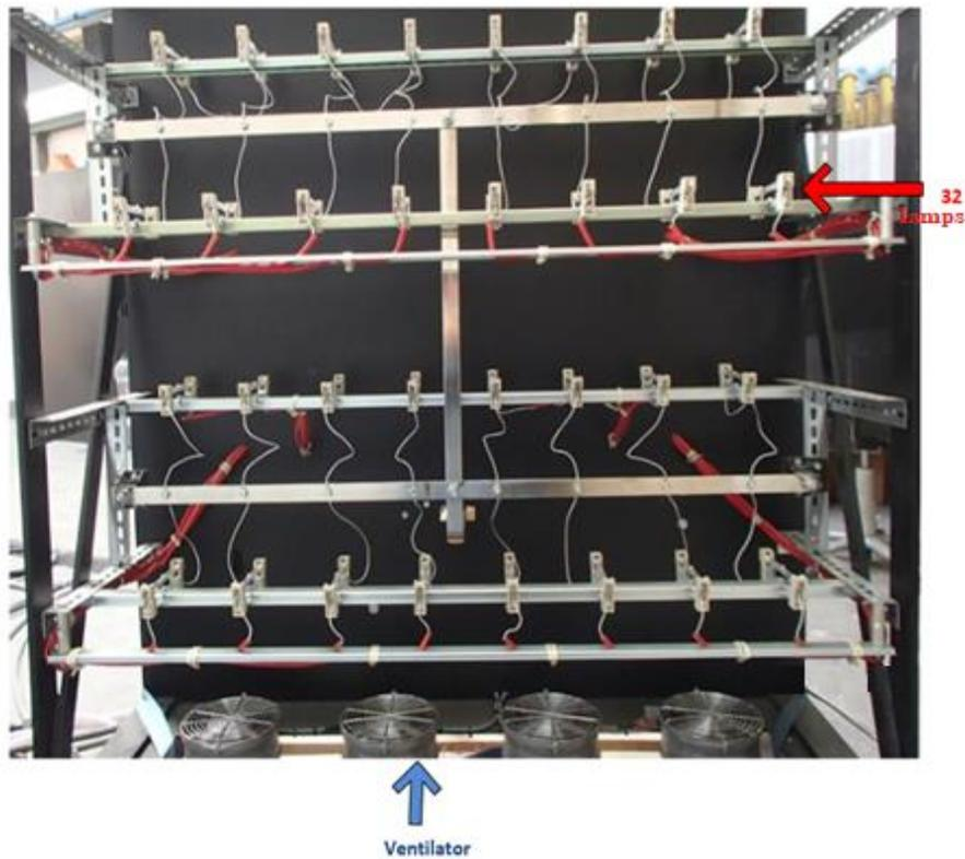
Fig. 4.21: Back of the variable load resistor
