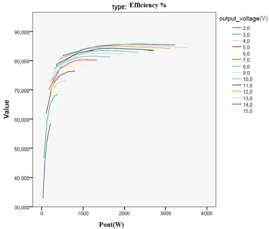
Fig. G.12: Efficiency vs Pout
