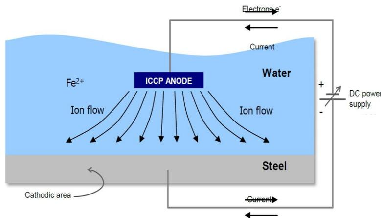
Fig. 1.2: Cathodic protection by impressed current
