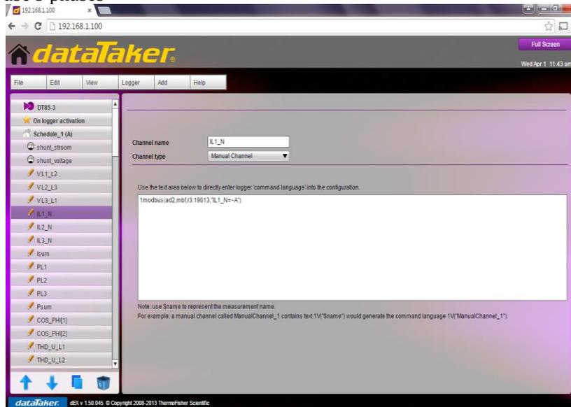
Fig. 4.18: Modbus address of phase current
