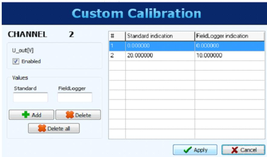
Fig. 4.11: Custom Calibration - for the output voltage
