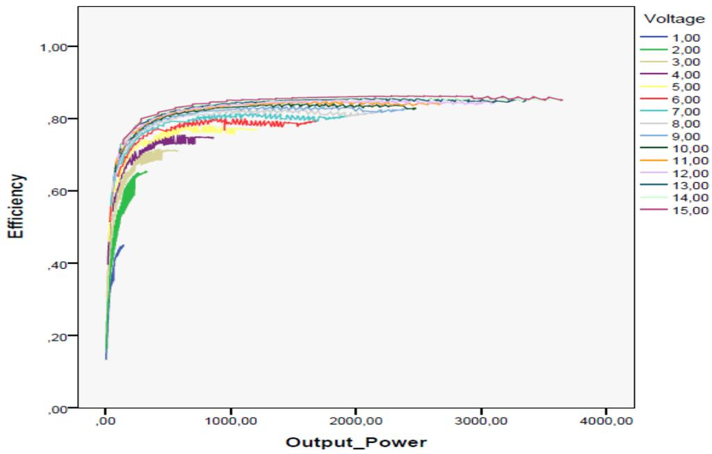
Fig. I.8: Power output vs efficiency
