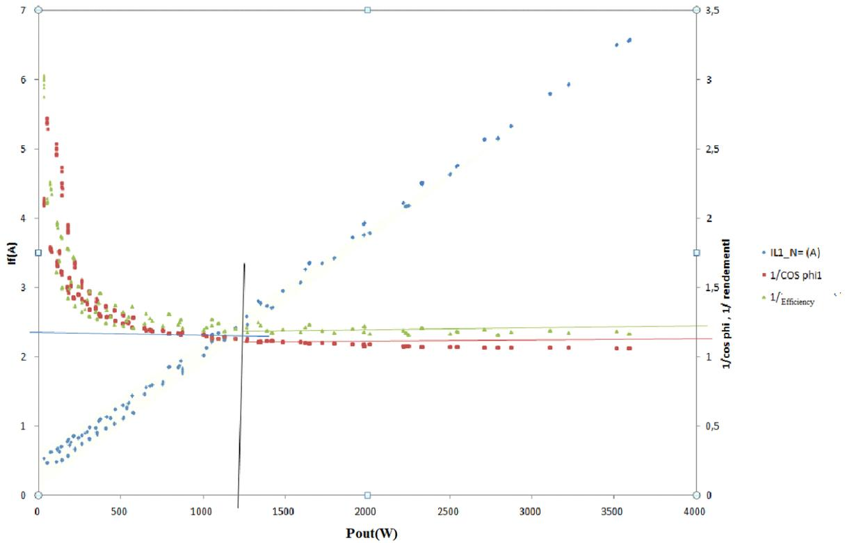
Fig. H.3: The relationship between power output, Cos phi and efficiency
