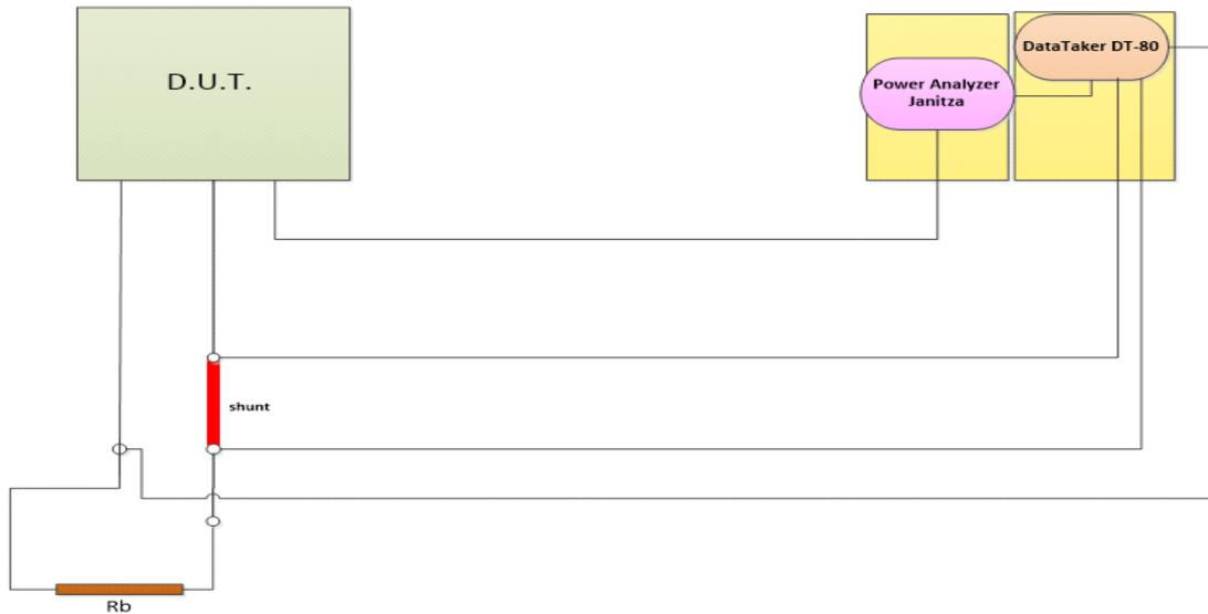
Fig. G.1: Block diagram of the tests of test 2
