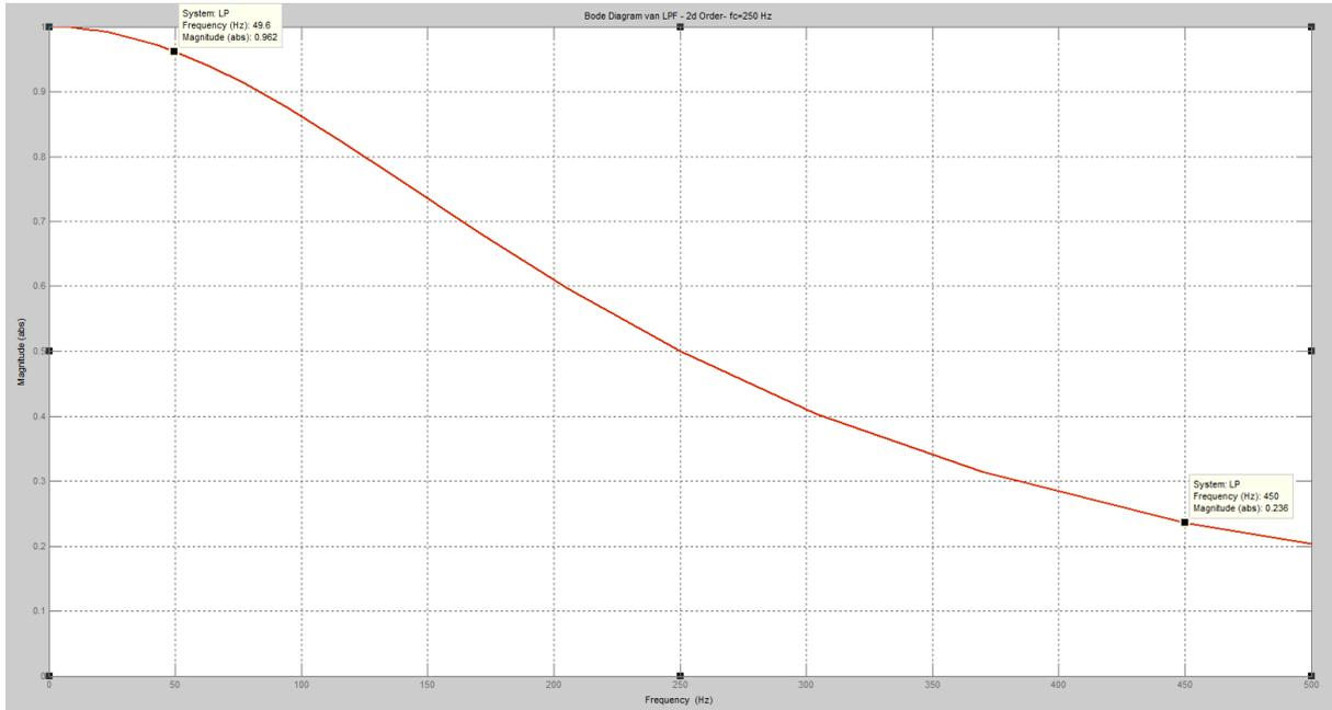
**Fig. 6.13: Bode diagram of LPF - 2d order - fc=250 Hz**
