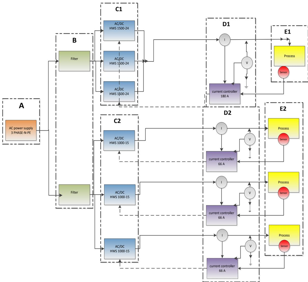
Fig. 3.1: Electrical diagram of measuring and control box of ICCP
