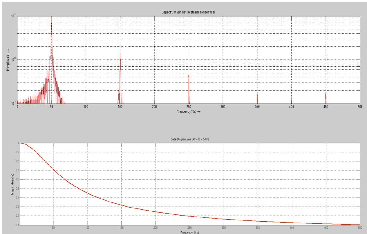
Fig. 6.9: Spectrum of current harmonics without filter and bode diagram of LPF -  $f_c=50$  Hz
