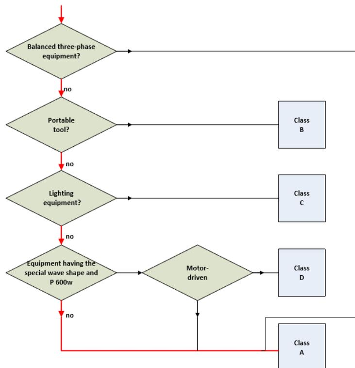
Fig. 2.1: Determine the scheme for the class
