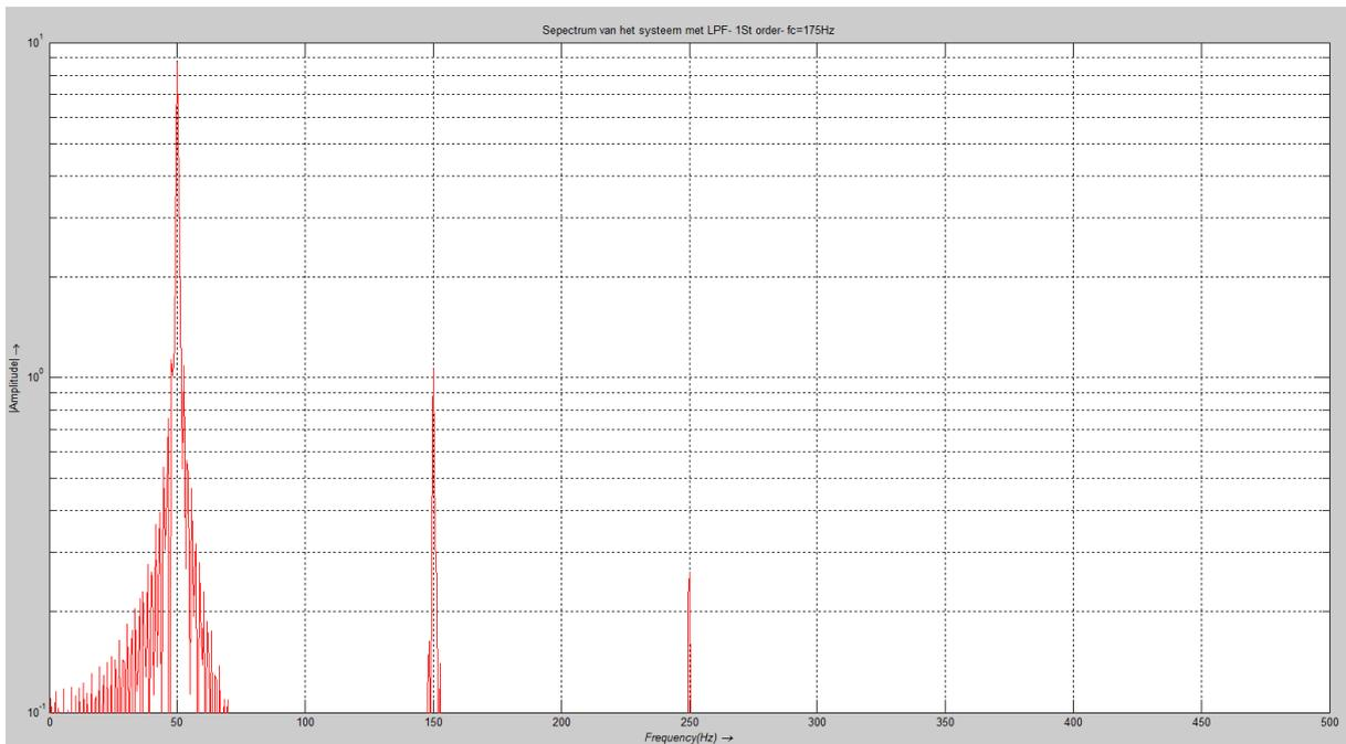
Fig. 6.12: Spectrum of current harmonics of the system with LPF  $f_c=175$  Hz
