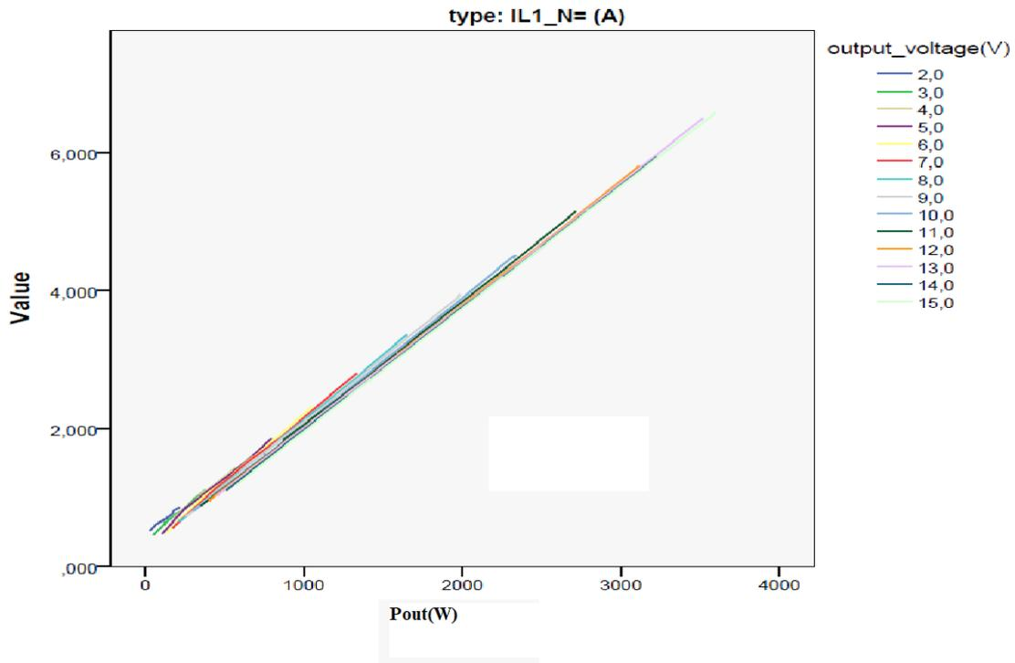
Fig. G.2: The output power vs the input current
