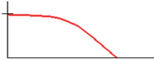
Fig. 6.1: Low -pass filter
