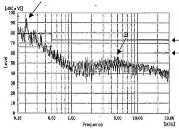
Fig. C.3: Electric magnetic interference properties For HWS 1500-24
