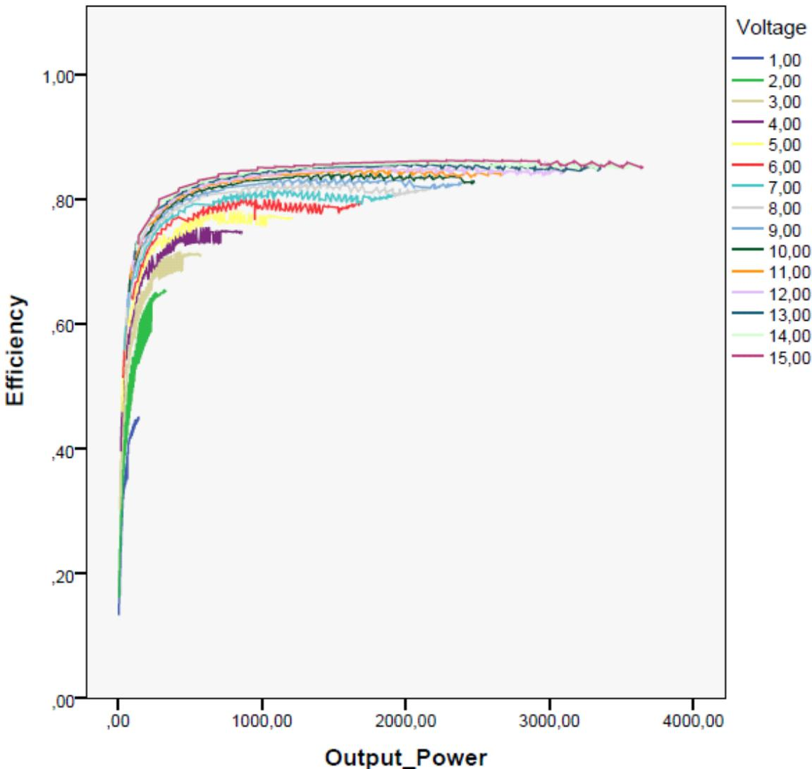
Fig. I.4: The power output (W) vs efficiency
