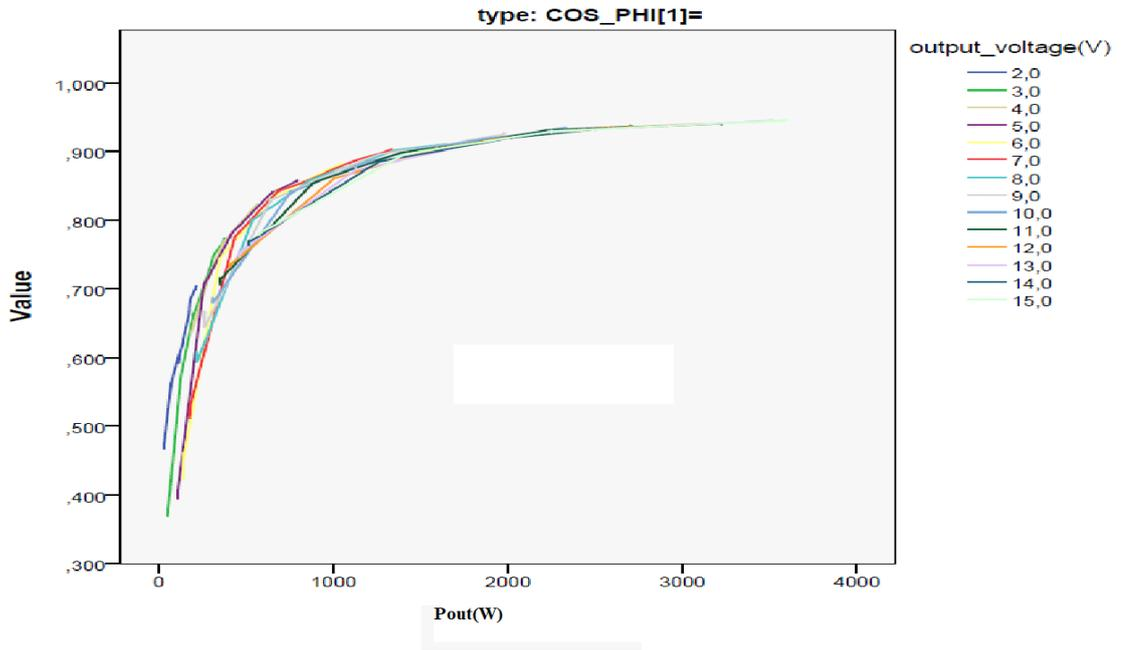
Fig. G.5: Cos phi vs Puit for phase 1
