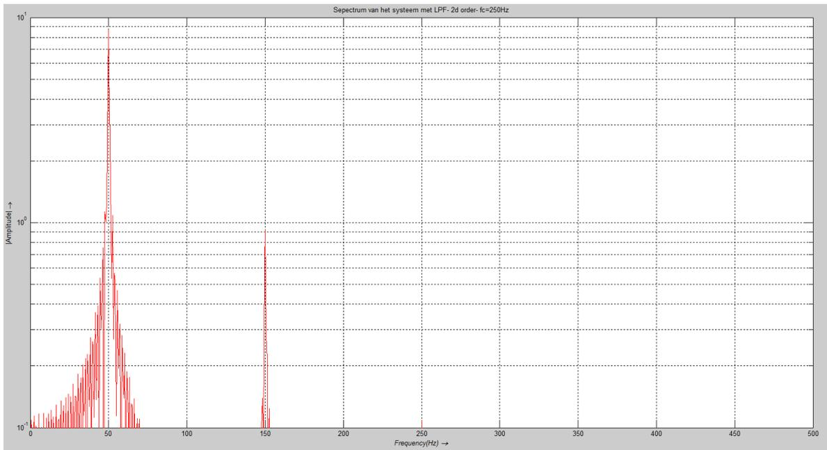
**Fig. 6.14: Spectrum of current harmonics of the system with LPF - 2d order fc=250Hz**
