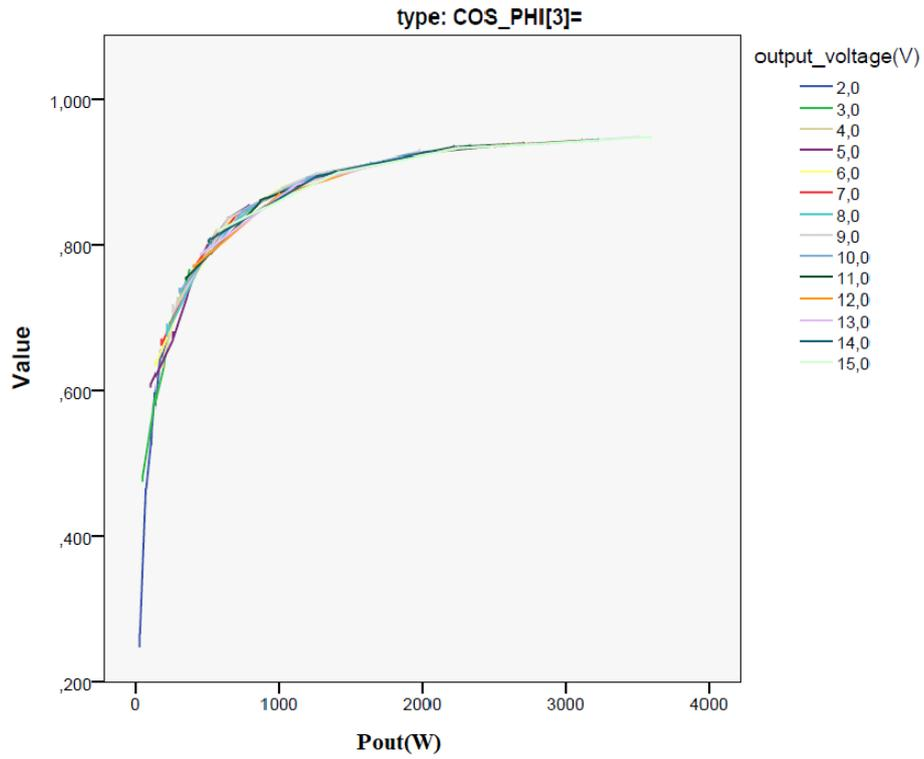
Fig. G.7: Cos phi vs Puit for phase 3
