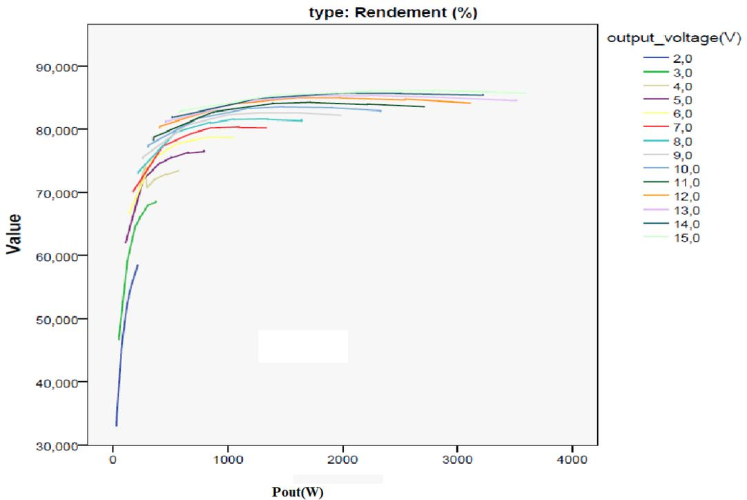
Fig. H.1: Pout VS efficiency
