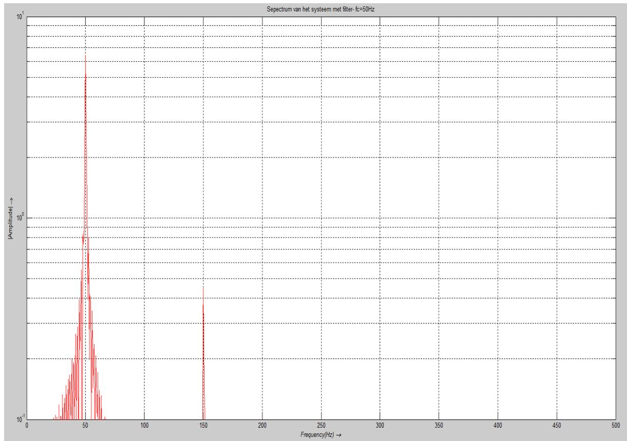
Fig. 6.10: Spectrum of current harmonics of the system with LPF  $f_c=50\text{Hz}$
