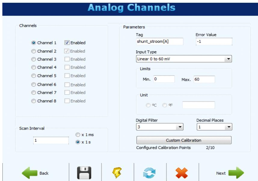
Fig. 4.8: Analog Channels Configuration- shunt current
