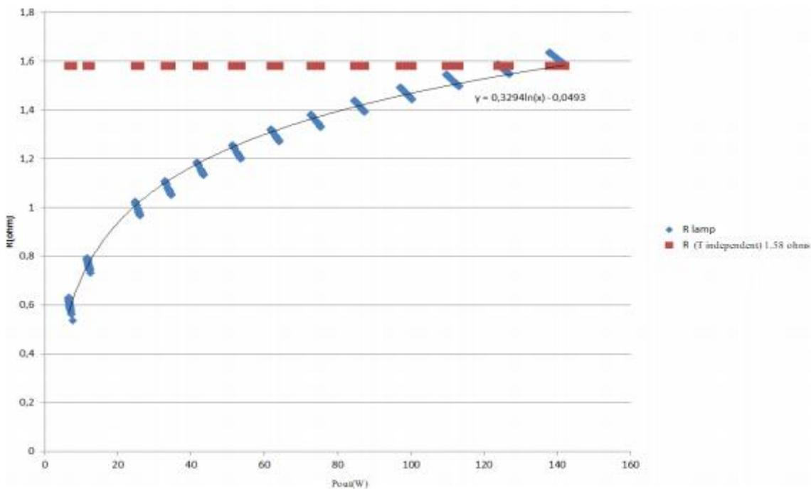
Fig. 4.34: Pout VS R-lamp
