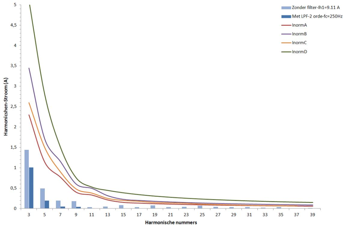
Fig. 6.6: Compare between harmonic current with and without filter
