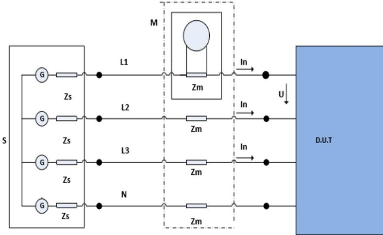
Fig.D.2: Measurement method of the harmonic currents of the test equipment (DUT0)
