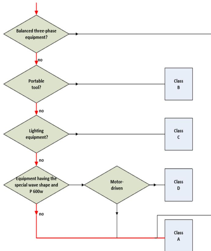
**Fig.D.1: scheme for determining the class**
