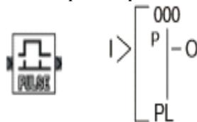
Fig. 4.27: " PL pulse-edge" function block
