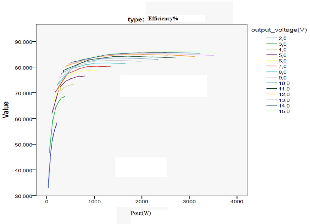
Fig. G.4: Power Output VS Efficiency
