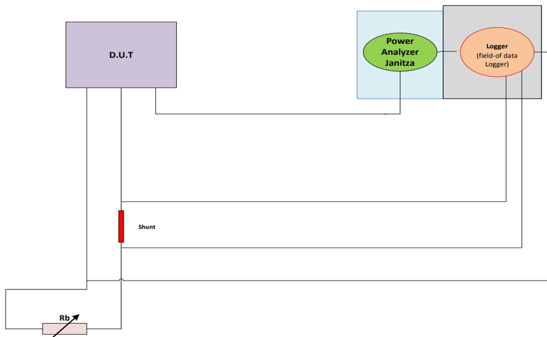
Fig. 4.1: Block diagram for ICCP
