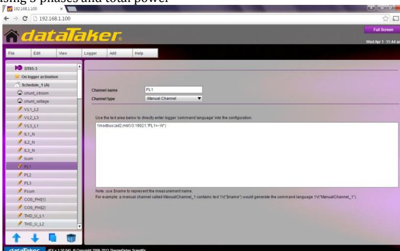
Fig. 4.19: Modbus address of phase power
