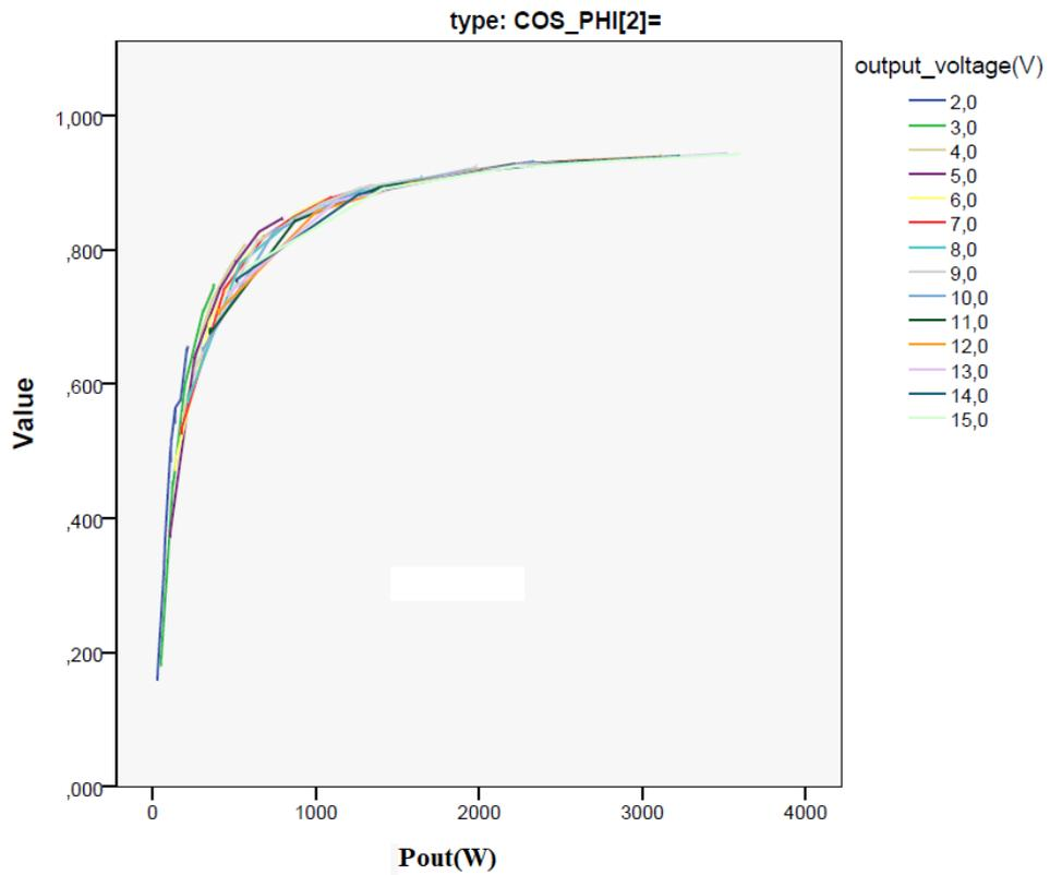
Fig. G.6: Cos phi vs Pout for phase 2
