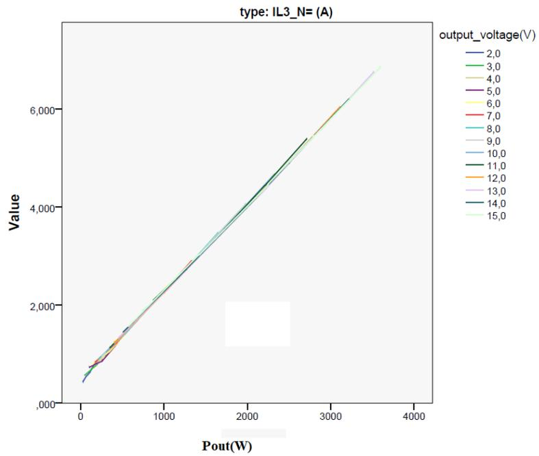
Fig. G.10: I fase vs Puit for phase 3
