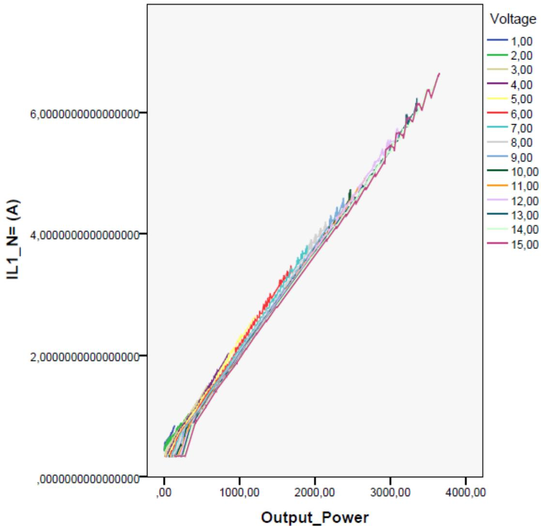
Fig. I.2: The output power(W) vs the input current(A)
