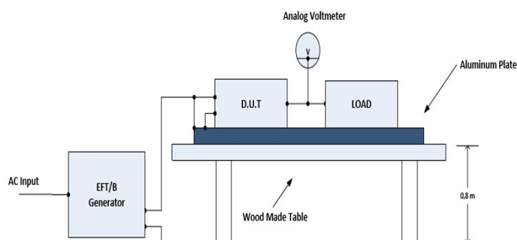
Fig. B.1: Guided Failure Test
