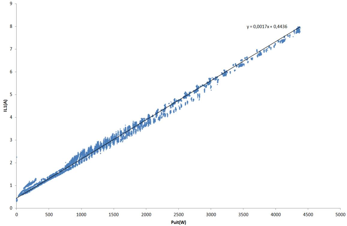
Fig. 5.6: Input Current VS Output Power
