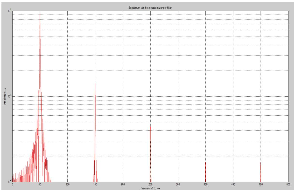
Fig. 6.7: Spectrum of current harmonics of the system without filter
