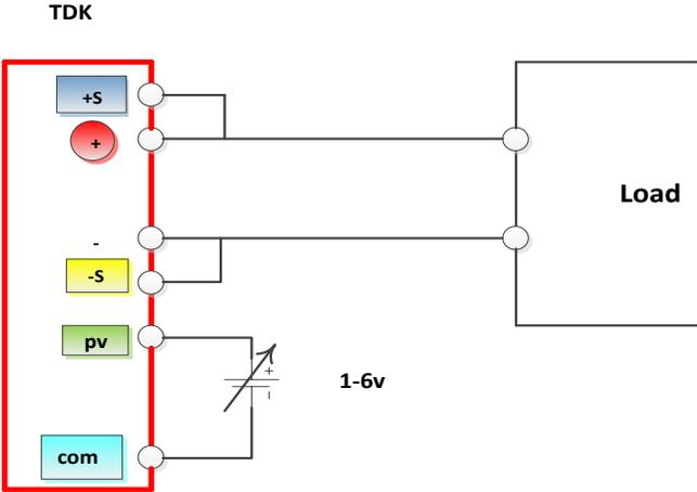
Fig. 3.4: Connection of the output voltage to external control
