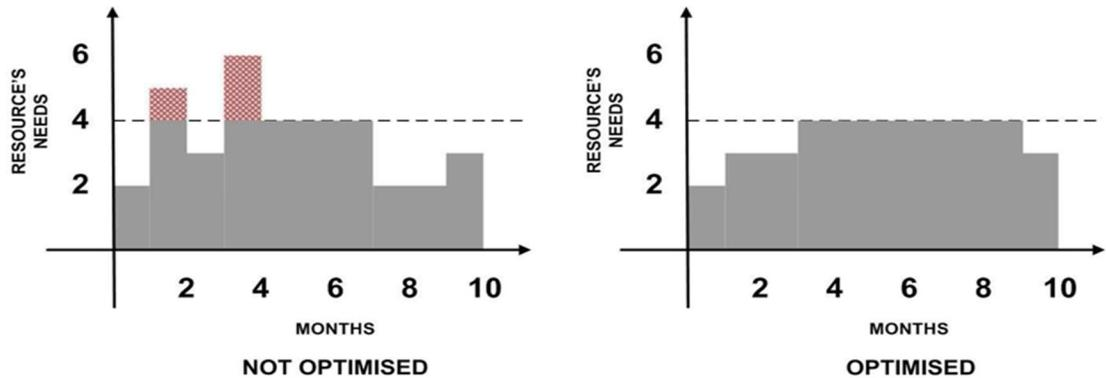
Fig 10: Construction Activities Load Diagrams, CIOB (The Chartered Institute of Building).
