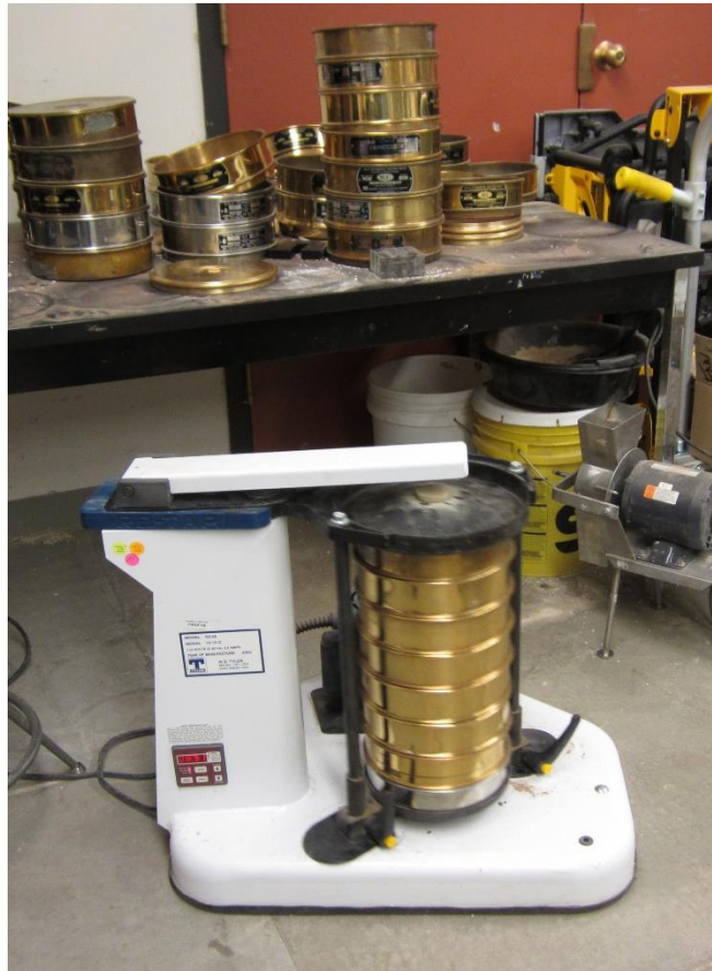
Figure 16: Sieve shaker with a stack of various sieve sizes containing testing range soil.
