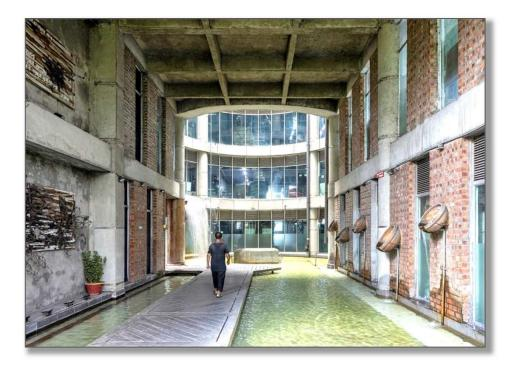
*Pic 4.44:* Designed layout of water inside the compound keeps the environment naturally cool (*Ref 4.72*)
