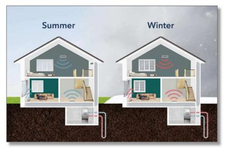
*Pic. 3.8*: Picture showing the concept how geothermal heating can help keep a house interior cool in summer as well as warm in winter. (Ref. 3.8)
