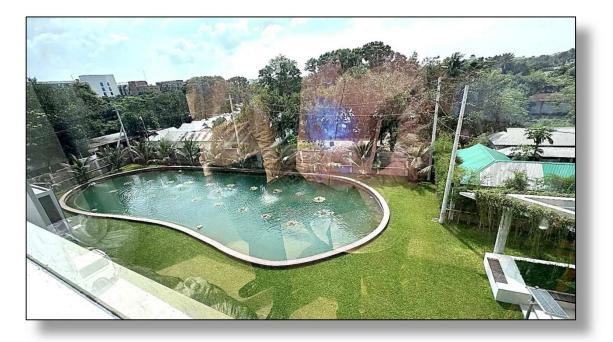
Pic 5.4.22: Rainwater reservoir collects rainwater and the water is treated for reuse. (Ref:ss
