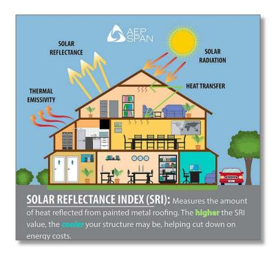
Pic. 3.1: Building roofs covered with light-reflecting materials or paints and SRI Index (Ref 3.17)
