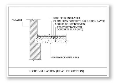
*Dia. 5.4.3:* Concept of laying patent stone as insulation on top of roof slab during construction of the building (Ref:ss)
