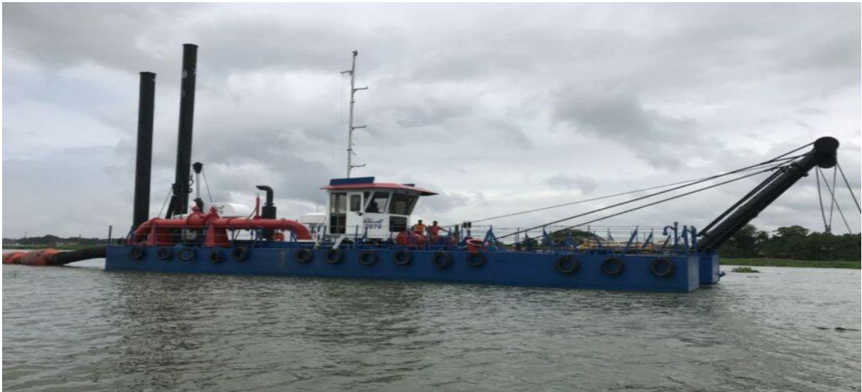
Figure 2-5: Ellicott dredger (Dragon)-Active in the Padma River
